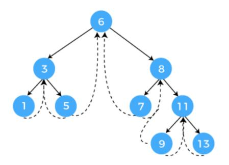
In two-way threaded binary trees, a node's right link field is replaced by a thread that links to the node's inorder successor, and a node's left link field is replaced by a thread that points to the node's inorder predecessor.
