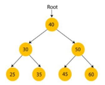
A binary search tree organizes its elements in a specific order. According to this structure, the value of a left node in a binary search tree must be less than the value of its parent node, while the value of a right node must be greater than that of its parent node. This rule is recursively applied to both the left and right subtrees of the root node.
